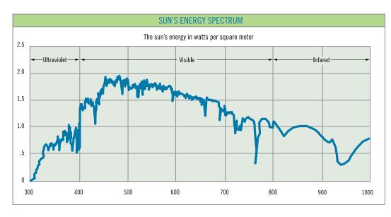
Because Tdw-ISO represents damage caused by both UV and visible wavelengths, it is a more accurate tool<sup>1</sup> for assessing potential fade resistance than the total UV transmittance measure that was (and is) traditionally used by many window manufacturers.
